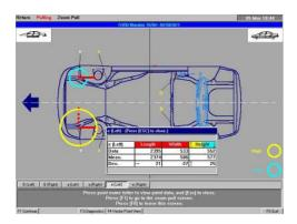
Double clicking on the vehicle image in the measurement results screen, brings up a larger image in a window which can be redimensioned and moved around on the screen. Here it has been placed below the table of the measurement points.
